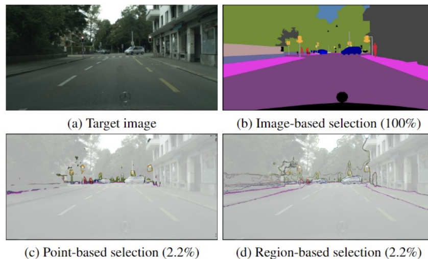
Figure 1. Illustration of different selection strategies. Image-based selection (e.g., MADA [41]) picks a few target samples and label the entire image, which is probably inefficient. Point-based selection (e.g., LabOR [54]) chooses scarce points about which the model is uncertain, while uncertainty estimation at point level is prone to lump pixels that come from particular categories. Our region-based selection asks for more annotations of regions with more categories as well as object boundaries in an effective way.
